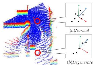
Figure 1: Degenerate surfel normal caused by a degenerate points shape.
