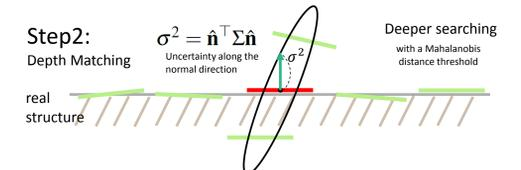
Figure 7: Proposed two staged matching algorithm. The step1 controls map resolution whereas the step2 reduces map noise by searching deeper along the LiDAR beam direction.
