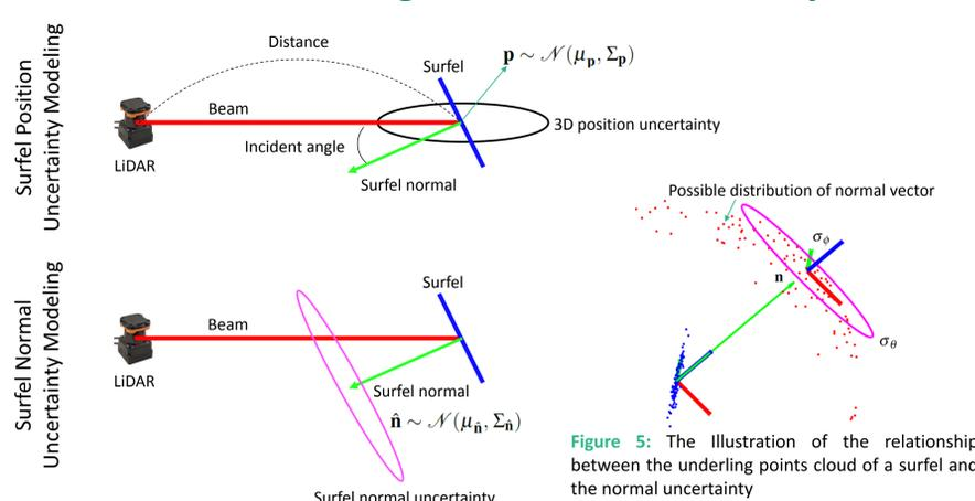
Figure 5: The Illustration of the relationship between the underlying points cloud of a surfel and the normal uncertainty
