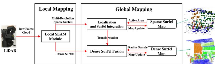
Figure 3: The proposed system is composed of two main stages. Local mapping stage processes the raw LiDAR data and creates local maps. The global mapping stage build a globally consistent map by merging them.
