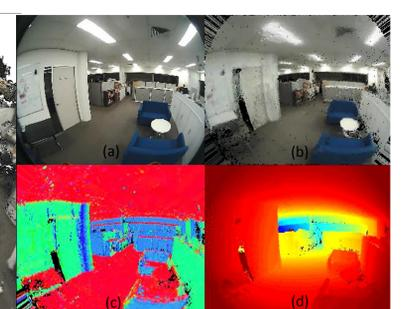
Figure 11: (a) Raw camera image of the office in the red circle. (b) Synthesized image from the surfel map. (c) Surfels map colored with normal direction. (d) Depth image.
