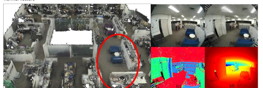
Figure 10: Reconstructed 3D surfel map of an office with a color fusion by camera images.
