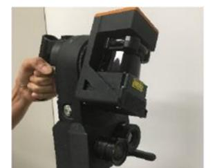
Figure 9: The experimental handheld 3D spinning LiDAR for mobile mapping.
